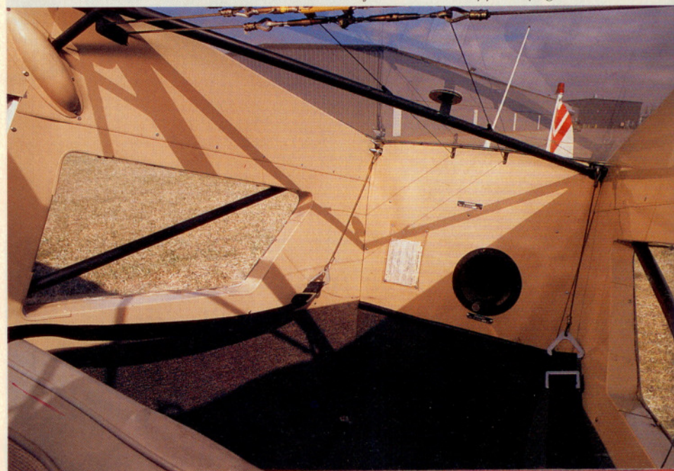
An expanse of plexiglass gives the Taylorcraft F21B's cramped cabin an open feel; the aircraft's steel tube framework, control cables, and elevator trim system are visible. Cockpit details include the elevator trim handle and visual fuel indicators (opposite page).
