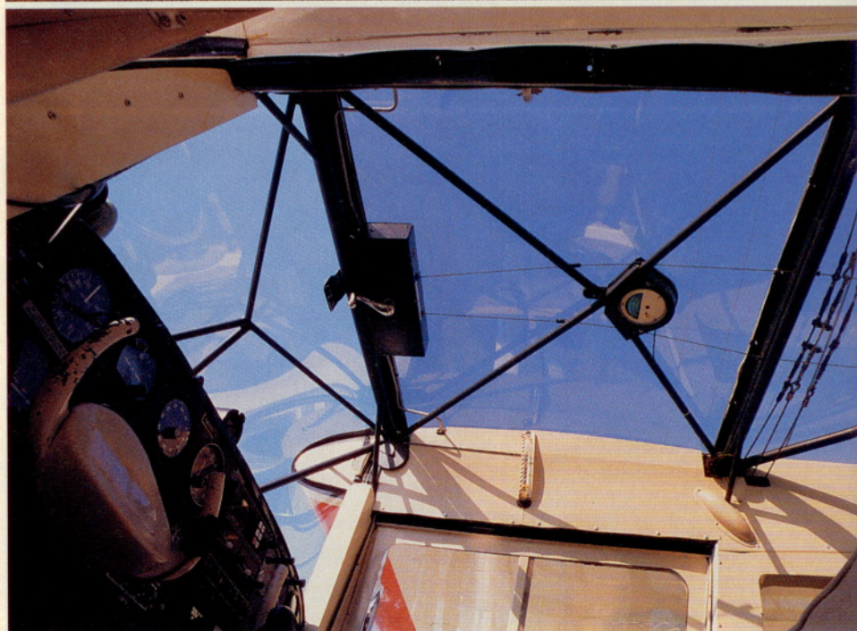
An expanse of plexiglass gives the Taylorcraft F21B's cramped cabin an open feel; the aircraft's steel tube framework, control cables, and elevator trim system are visible. Cockpit details include the elevator trim handle and visual fuel indicators (opposite page).
